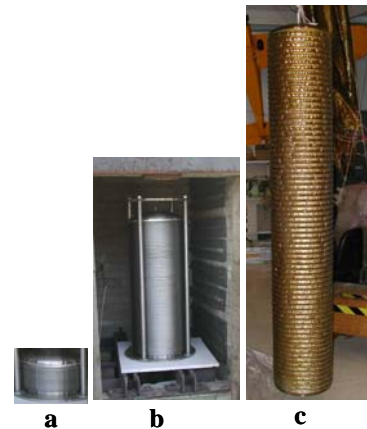
Figure 4. 0.35-m diameter metal bellows. a – at \Delta P = -84 mB, b – at \Delta P = 114 mB, c – at \Delta P = 630 mB after exposure to +460 C
